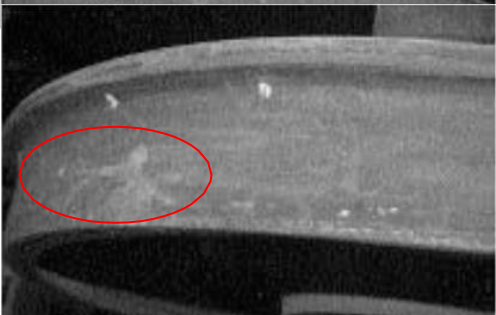
Fig. 9: Major irregular crushing of the edge of the tyred wheel rim
