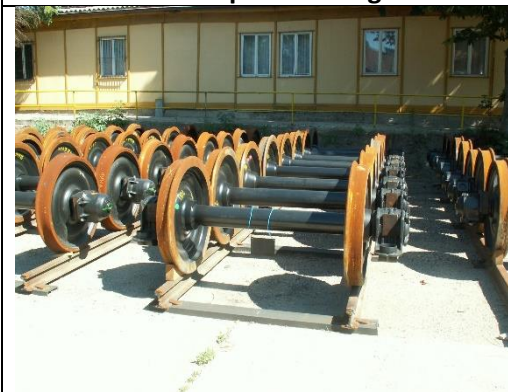
Photo 1: Storing on track using safety scotches
